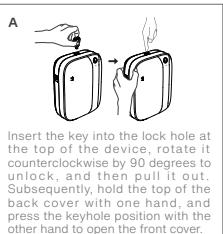
Insert the key into the lock hole at the top of the device, rotate it counterclockwise by 90 degrees to unlock, and then pull it out. Subsequently hold the top of the back cover with one hand, and press the keyhole position with the other hand to open the front cover.
