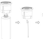
remove it. Next, replace it with a new atomizer core, and then reassemble all parts back into the device.
