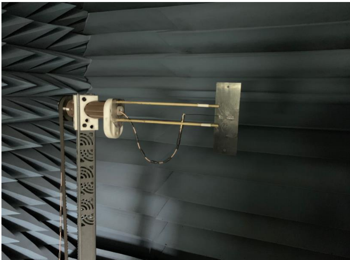
FIGURE4.1.3 ANTENNA LOADED WITH PC/ABS BLOCK OF 1.5 MM THICKNESS WITH OTA CHAMBER
