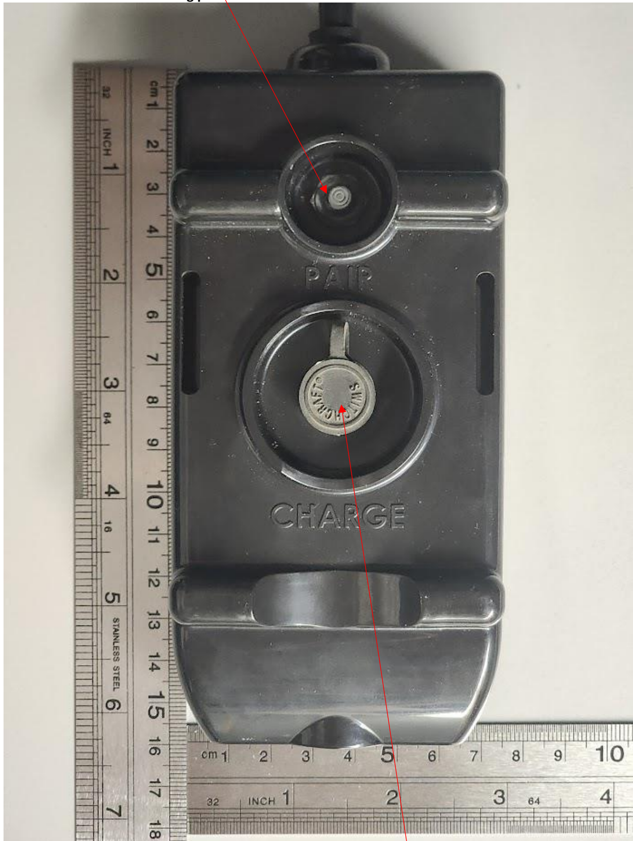
Battery Charging Port
