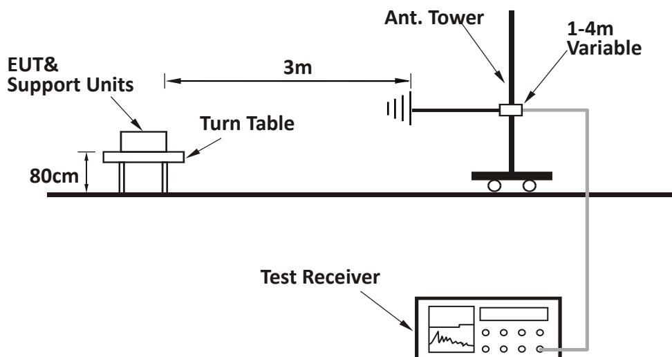
**TEST REPORT****For Radiated emission above 1GHz:**
