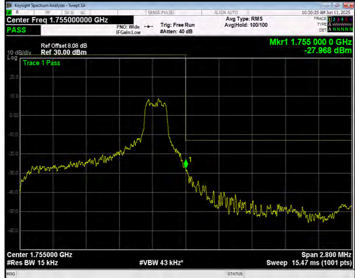
Band4 QPSK BW=1.4MHz Channel=20393 RB Size=1 Position=#Max NB Index=0
