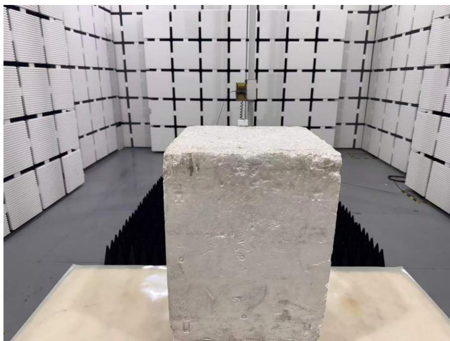
Set-up for Radiated Spurious Emission, Above 1GHz
