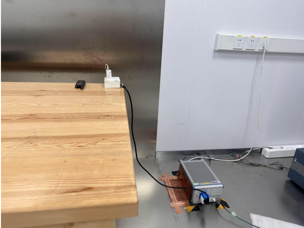
Radiated Emission Test View|(Below 1G)
