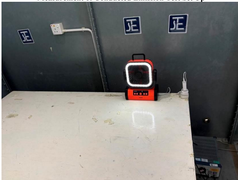
Measurement of Conducted Emission Test Set Up
