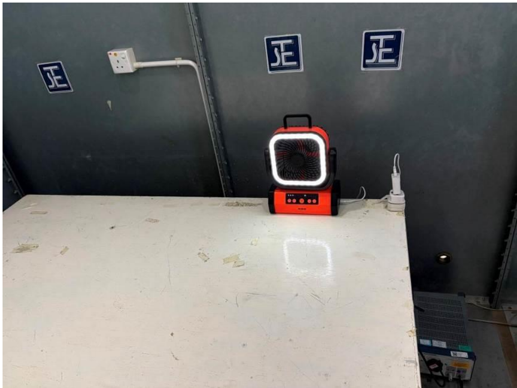
Measurement of Conducted Emission Test Set Up
