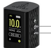
Press and hold power and decrease buttons together until the display show "PAIR" (Active time 20 seconds)
