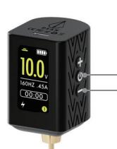
Need to delete the last record, press hold power and decrease buttons together, when display "PAIR" then press power button then it will display "DEL"
