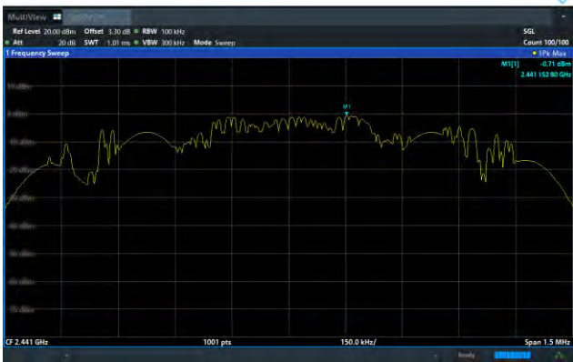
\pi/4 -DQPSK on Channel 39
