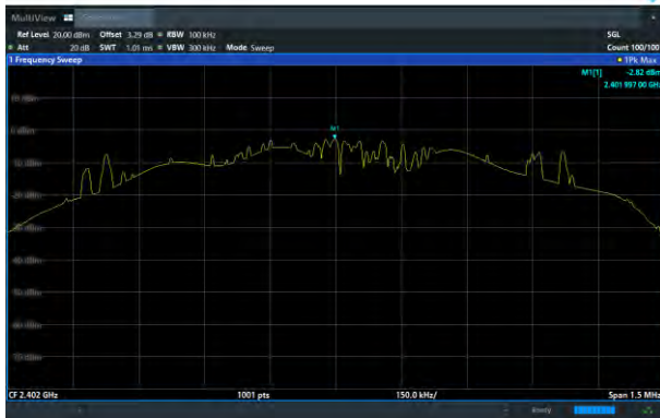
8DPSK on Channel 00
