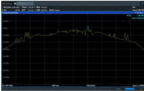
8DPSK on Channel 39
