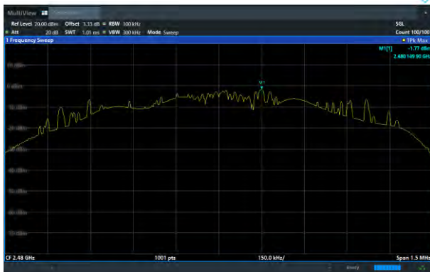
8DPSK on Channel 78
