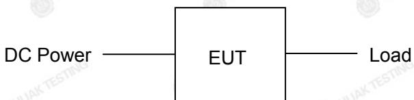
Operation of EUT during RF conducted testing:
