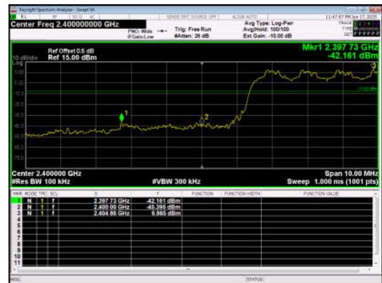
Out Of Band Emission(Left) \pi/4 DQPSK_2-DH5_Channel Hopping
