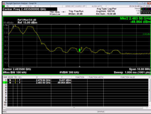
Out Of Band Emission(Right) GFSK_DH5_Channel Hopping
