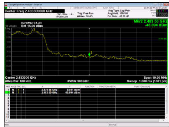
Out Of Band Emission(Right) \pi/4 DQPSK_2-DH5_Channel Hopping
