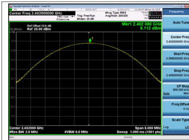
Peak Output Power 8DPSK_Channel 0
