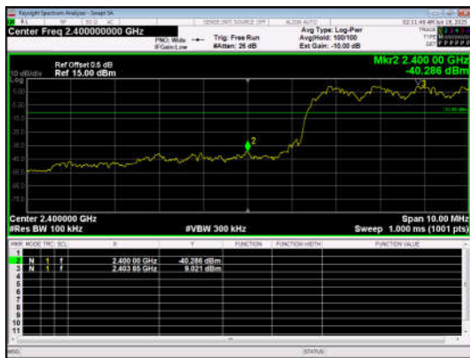
Out Of Band Emission(Left) 8DPSK_3-DH5_Channel Hopping
