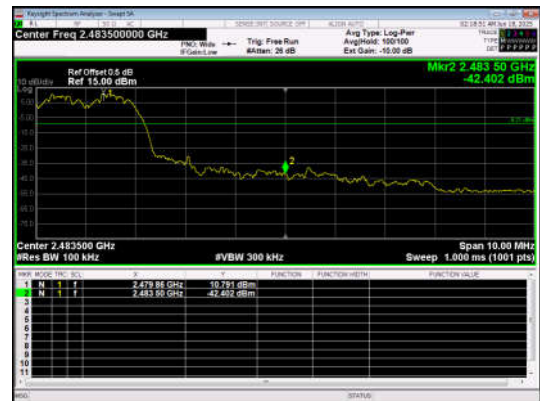
Out Of Band Emission(Right) 8DPSK_3-DH5_Channel Hopping
