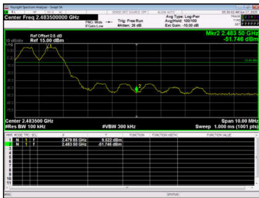
Out Of Band Emission(Right) GFSK_DH5_Channel Hopping
