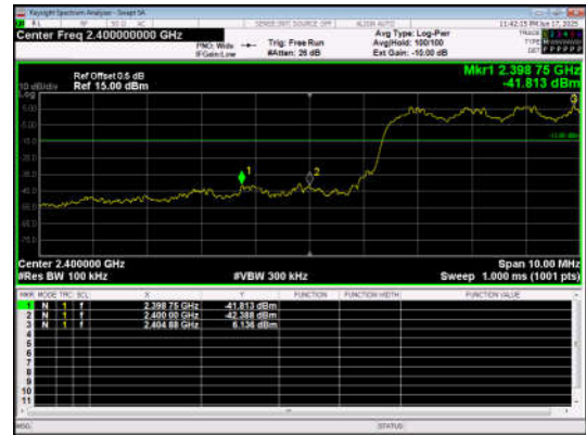
Out Of Band Emission(Left) \pi/4 DQPSK_2-DH5_Channel Hopping
