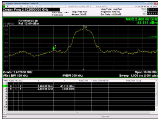
Out Of Band Emission 8DPSK_3-DH5_Channel 0
