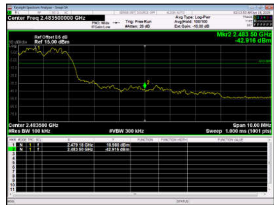
Out Of Band Emission(Right) 8DPSK_3-DH5_Channel Hopping
