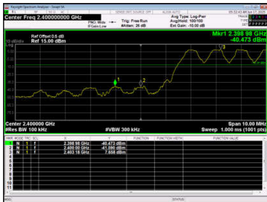
Out Of Band Emission(Left) GFSK_DH5_Channel Hopping
