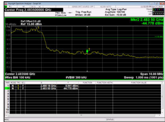
Out Of Band Emission(Right) \pi/4 DQPSK_2-DH5_Channel Hopping
