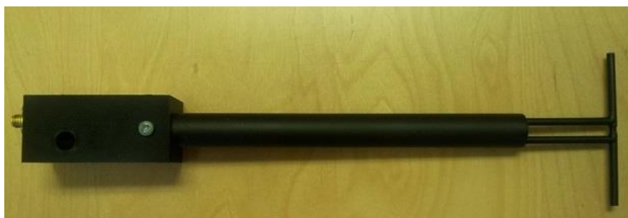
Figure 1 – MVG COMOSAR Validation Dipole
