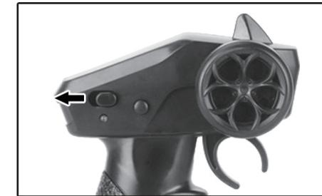
Turn on the power: Pull the power switch of the remote control car to the "ON" position, then turn on the power switch of the remote control. If the remote control operation indicator light is always on, the frequency binding is successful.
