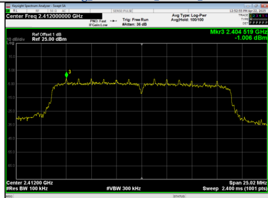
In-Band Reference Level IEEE 802.11n_Channel 1_20MHz_Antenna 0
