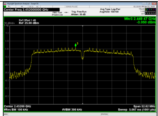
In-Band Reference Level IEEE 802.11n_Channel 9_40MHz_Antenna 0
