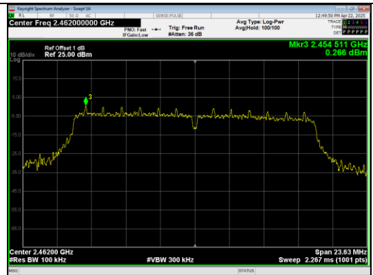
In-Band Reference Level IEEE 802.11g_Channel 11_20MHz_Antenna 0
