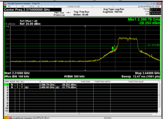
Out Of Band Emission IEEE 802.11g_Channel 1_20MHz_Antenna 0
