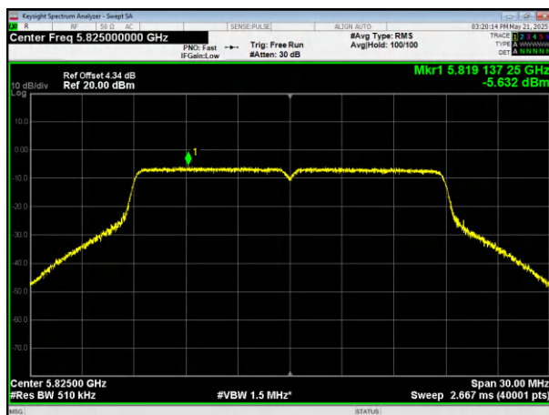
(802.11n20) PSD plot on channel 165
