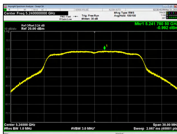
(802.11a) PSD plot on channel 48
