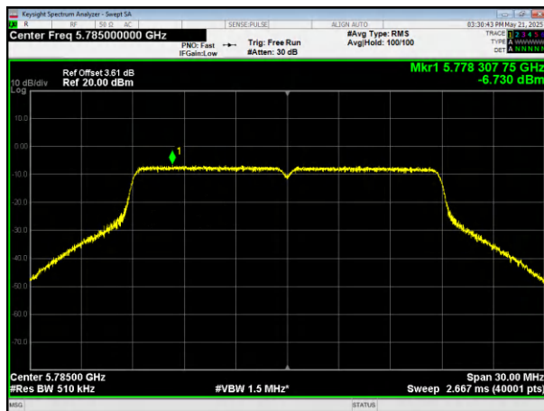
(802.11ac20) PSD plot on channel 157
