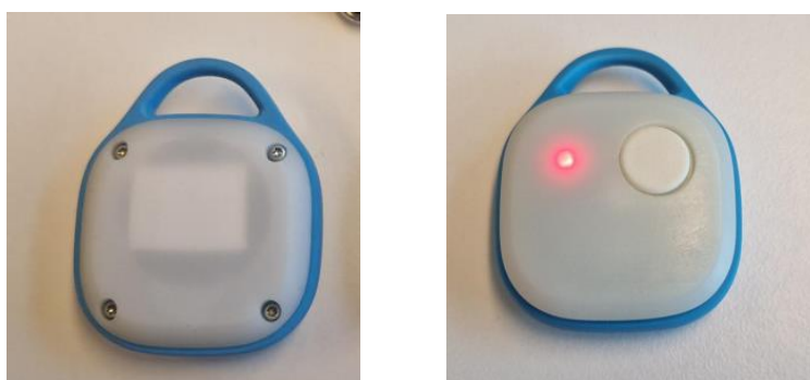
Figure 5. Tag with back cover closed. LED indicates power-on (if configured to do so).
