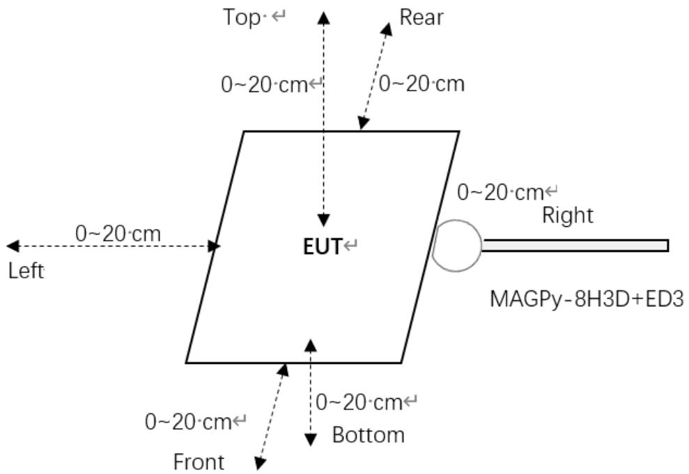
Note: tips mode of the test probe is used for 0cm measurement.
