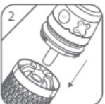
2. Align the head motor with the hole in the soft elastomer motor.
