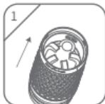
1. Place the elastomer in the cup and align the groove with the indicator sticker.
