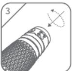
3. Turn counter clockwise to fix the head once the motor is fully inserted into the hole.
