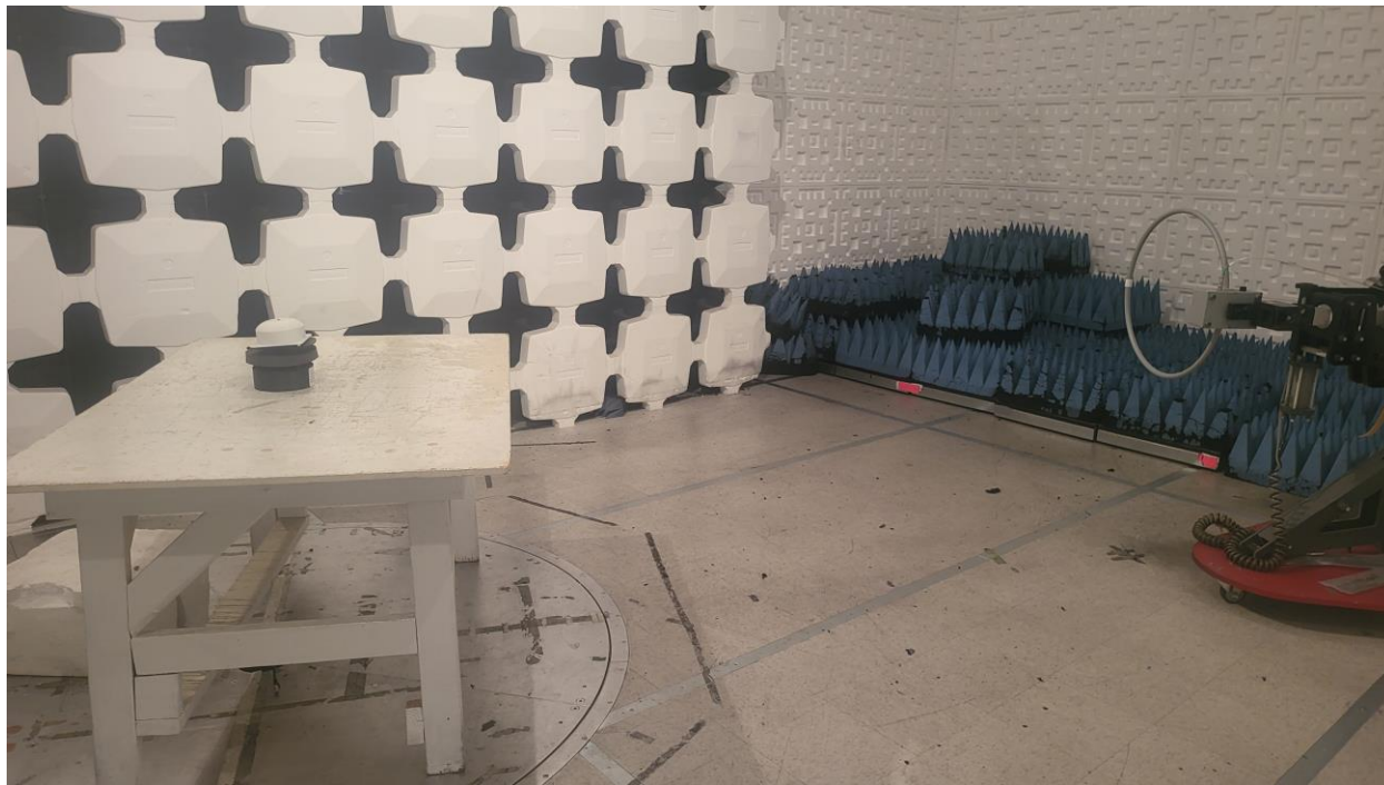
Figure 2. Radiated Emissions Test Setup, .15 MHz to 30 MHz
