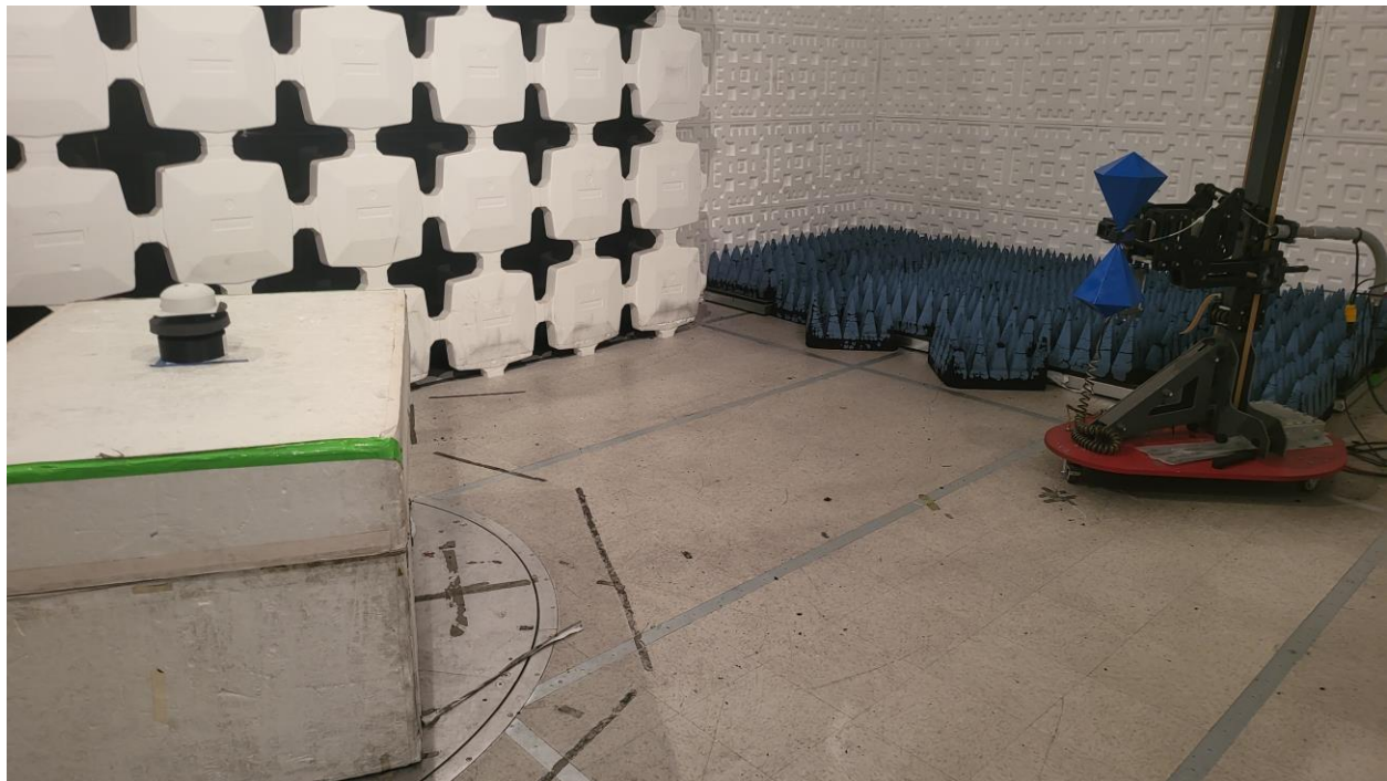
Figure 3. Radiated Emissions Test Setup, 30 MHz to 1000 MHz
