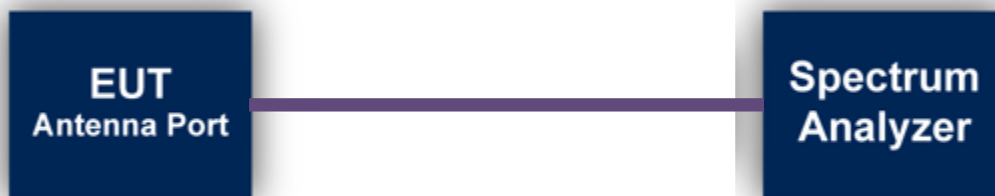
Figure 2: Direct Connection at the Antenna Port Test
