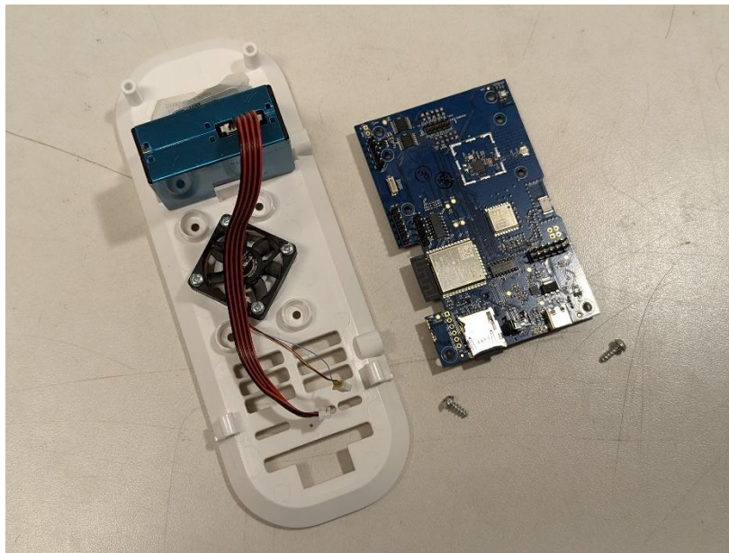
Photograph 16: PCB Placement in Enclosure Rear Showing EUT Unfastened
