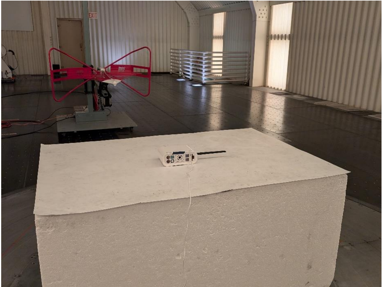
Photograph 5: Antenna Horizontal Placement
