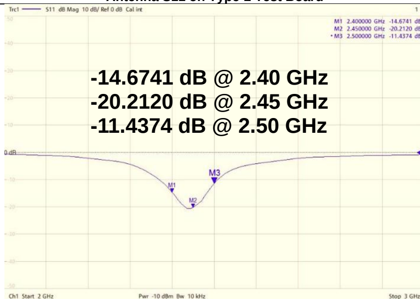
Antenna VSWR on Type-2 Test Board
