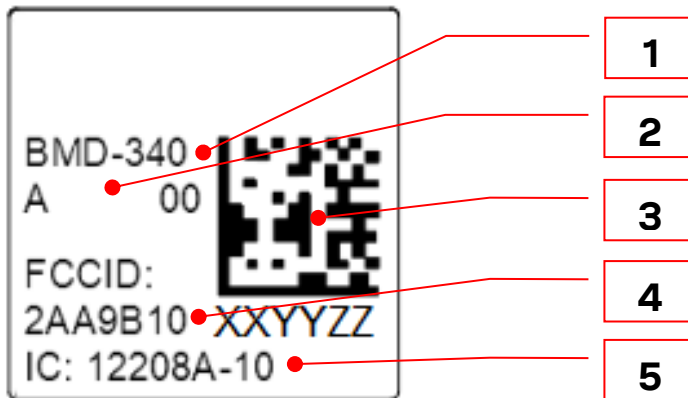
Figure 13: Module marking for type number BMD-340-A-R-00
