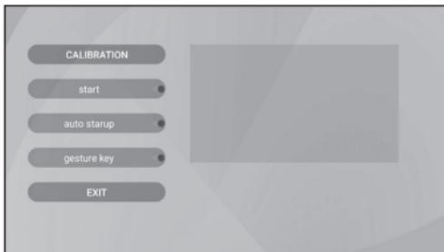
The calibration first performs a test of the proper functioning of the integrated camera by projecting a special pattern.
