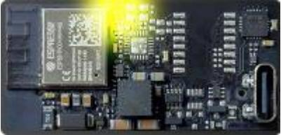
A photograph of the printed circuit board (PCB) of the Scandoc nano OP device. The board is dark blue/black and densely populated with electronic components, including a central microcontroller, various chips, and connectors. A small yellow LED is visible on the right side. The board is mounted on a dark, rectangular plastic housing. |
