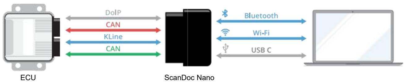
There are five types of adapters. Each works only with its own group of car brands. All five adapters have the same circuit and printed circuit board. The difference is in the switching of the CAN interface pins of the OBDII connector and the presence or absence of an Ethernet interface for communication with the car.
