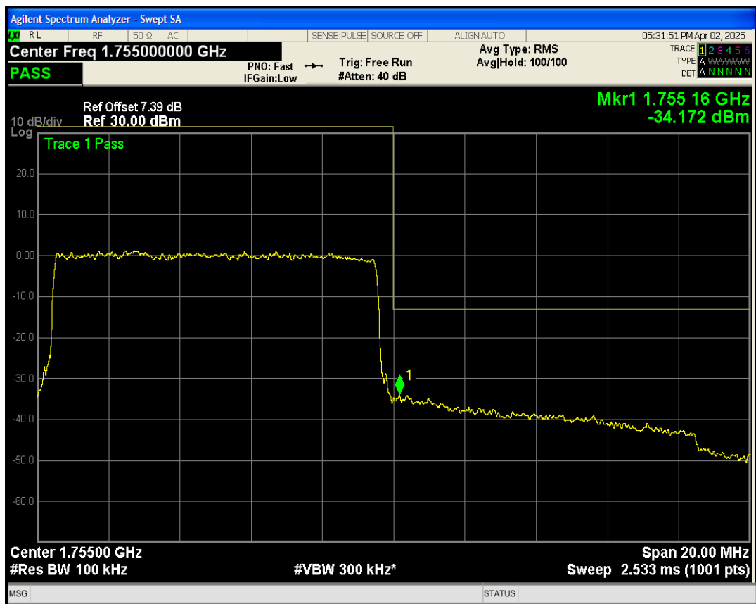
Band4 QPSK BW=15MHz Channel=20025 RB Size=75 Position=#0
