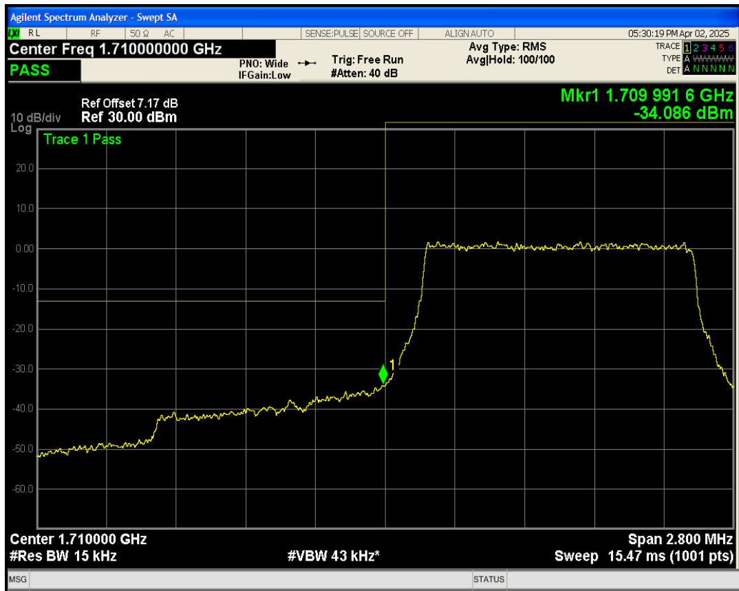
Band4 QPSK BW=1.4MHz Channel=20393 RB Size=6 Position=#0
