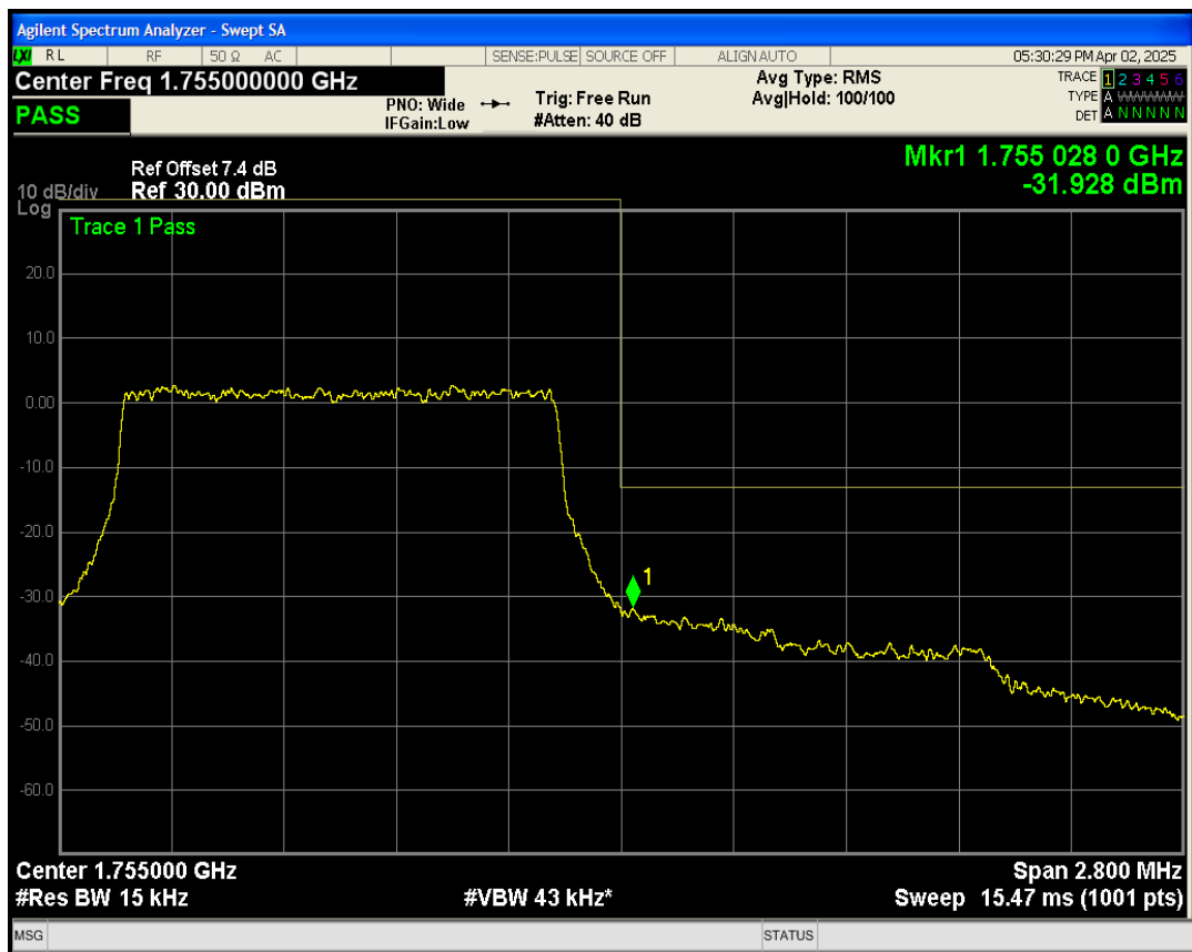
Band4 QAM16 BW=1.4MHz Channel=19957 RB Size=6 Position=#0
