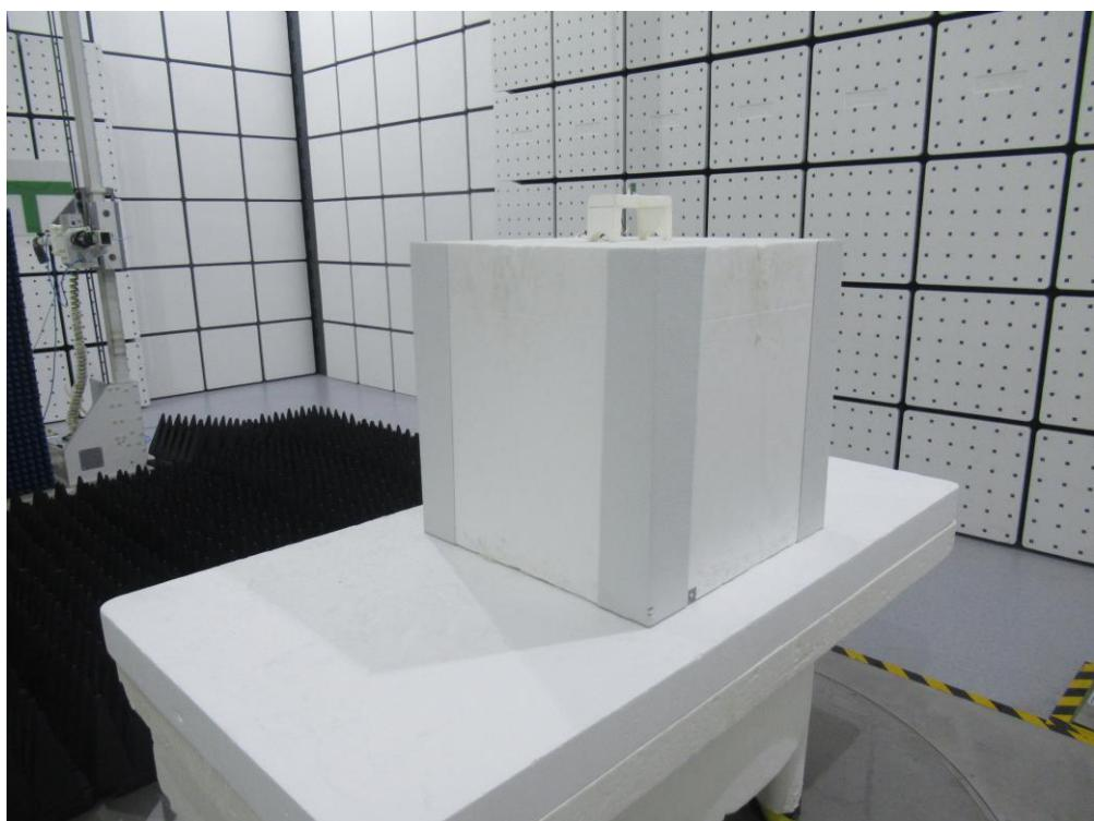
Description: Radiated Spurious Emissions Test Setup for 9kHz ~ 30MHz (PCB Antenna – External)
