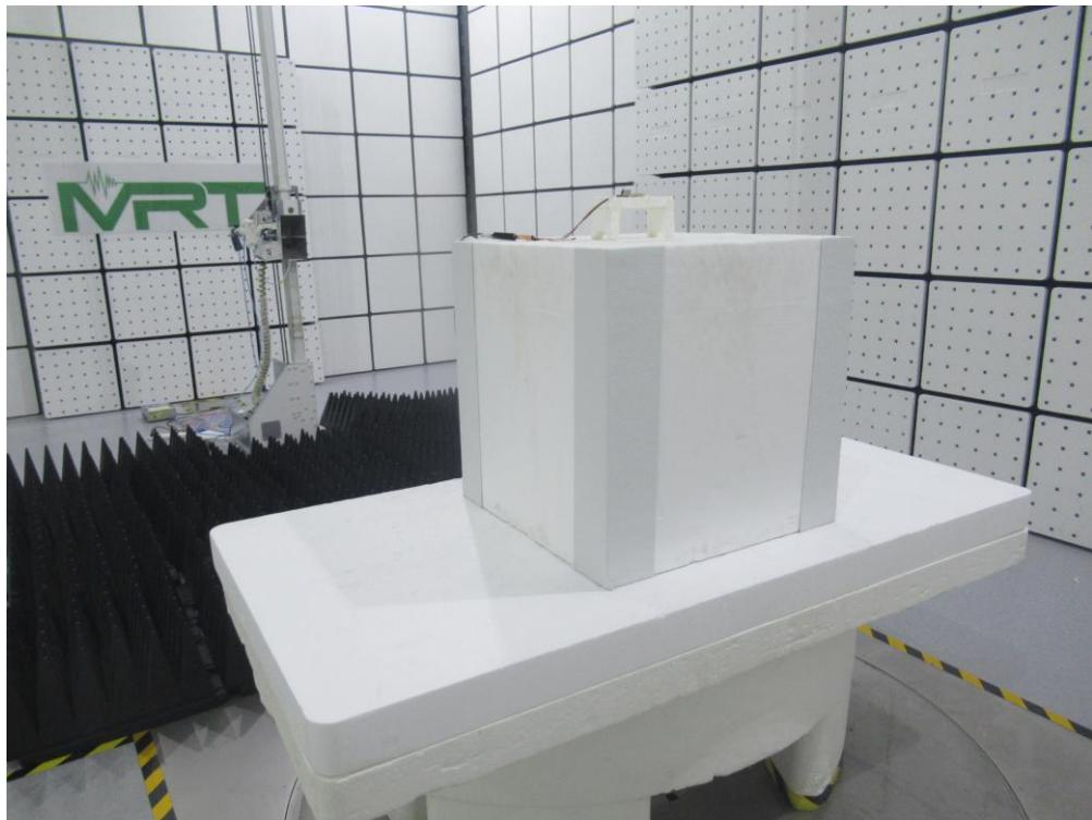
Description: Radiated Spurious Emissions Test Setup for above 18GHz (PCB Antenna – External)
