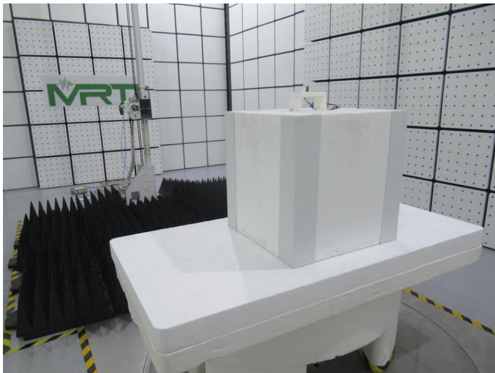
Description: Radiated Spurious Emissions Test Setup for above 18GHz (PCB Antenna – On board)
