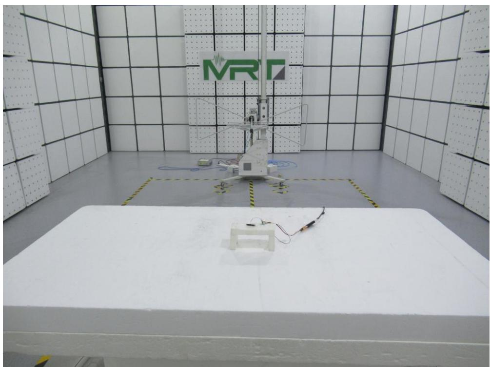
Description: Radiated Spurious Emissions Test Setup for 1GHz ~ 18GHz (PCB Antenna – External)
