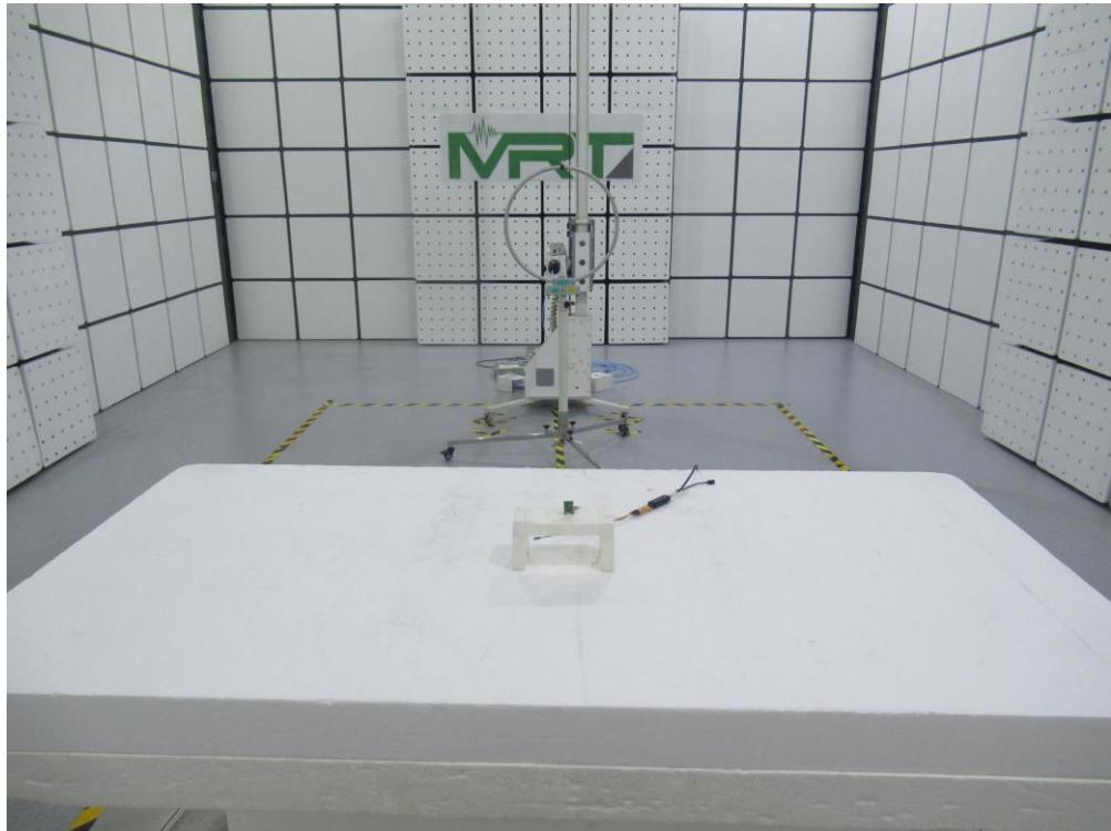
Description: Radiated Spurious Emissions Test Setup for 30MHz ~ 1GHz (PCB Antenna – On board)
