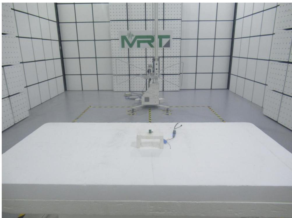
Description: Radiated Spurious Emissions Test Setup for 1GHz ~ 18GHz (PCB Antenna – On board)
