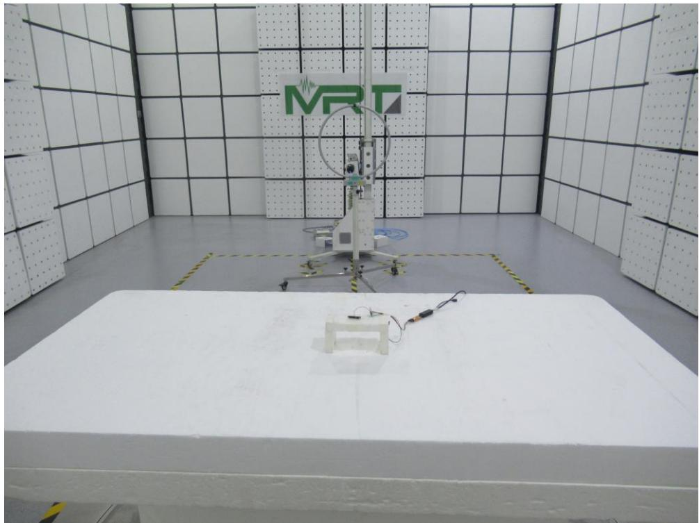
Description: Radiated Spurious Emissions Test Setup for 30MHz ~ 1GHz (PCB Antenna – External)
