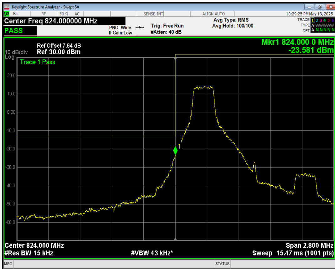
Band5 QPSK BW=1.4MHz Channel=20407 RB Size=6 Position=#0
