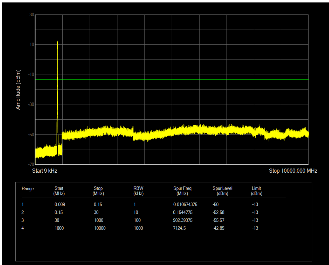
Band5 QAM16 BW=3MHz Channel=20525 RB Size=15 Position=#0
