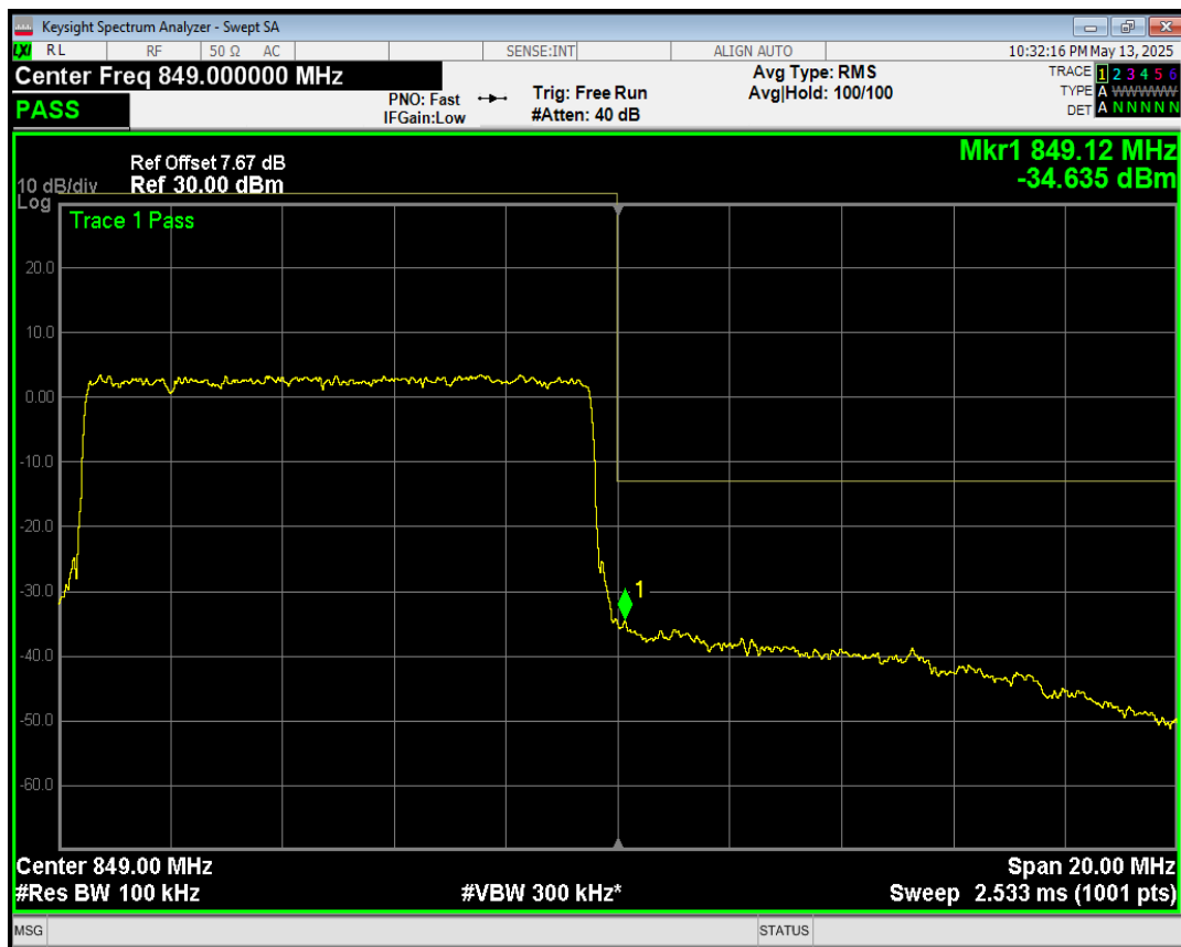
Band5 QAM16 BW=5MHz Channel=20425 RB Size=1 Position=#0
