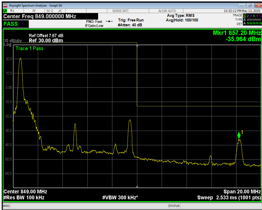
Band5 QAM16 BW=10MHz Channel=20600 RB Size=50 Position=#0
