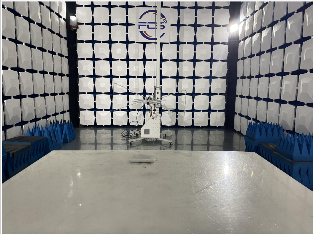
Above 1GHz for radiated emission test setup
