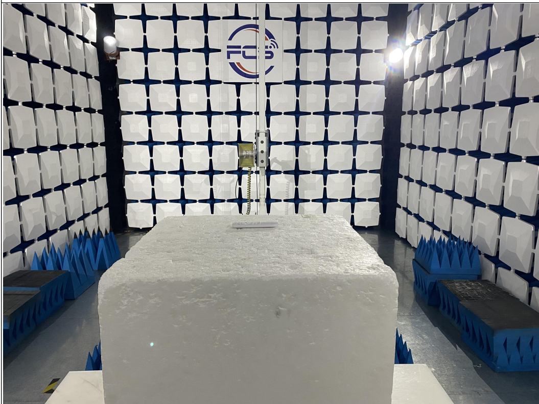
Above 1GHz for radiated emission test setup
