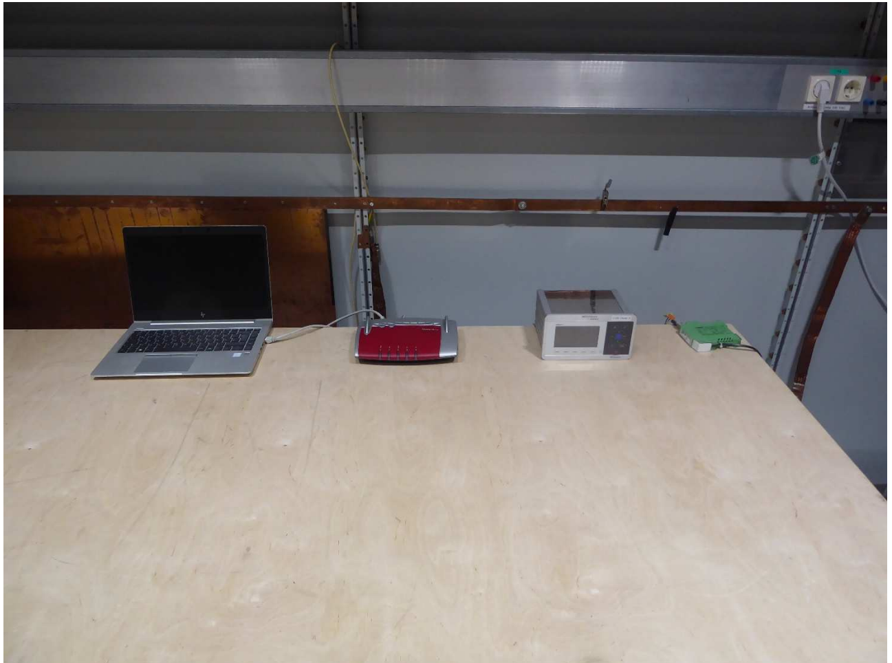
Test setup AC powerline conducted EUT 2 (24V DC)
