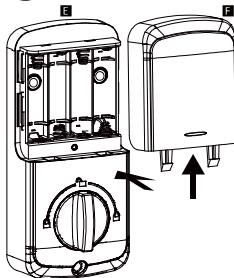
Press the battery cover and pull the cover up.
