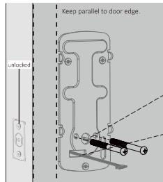
Secure the mounting plate with the screws I.
