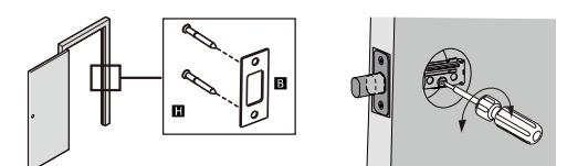
IMPORTANT: Make sure the hole in the door frame is drilled at a minimum of 1" (25 mm) deep.
