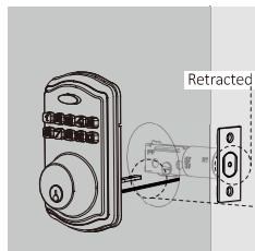
1. Before installation, make sure the latch is fully retracted (in the unlocked position).
