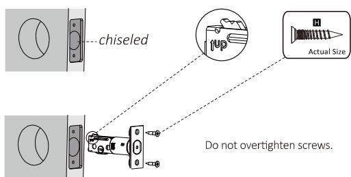
Do not overtighten screws.
