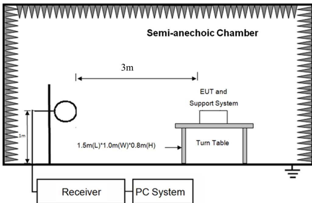
Test Setup Diagram for 30MHz~1GHz
