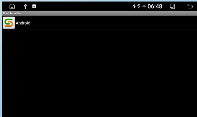
Connect the USB device containing the boot animation to the USB/SD of the box ->Open the [Boot Animation] application ->Drop down menu ->Click menu button ->Enter password, and the animation package in the USB device will automatically synchronize
