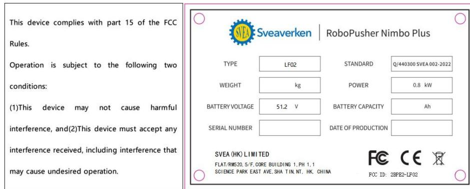
Specifications: The label shall be securely affixed to a permanently attached part of the device, in a location where it is visible or easily accessible to the user, and shall not be readily detachable. The label shall be sufficiently durable to remain fully legible and intact on the device in all normal conditions of use throughout the device's expected lifetime.
