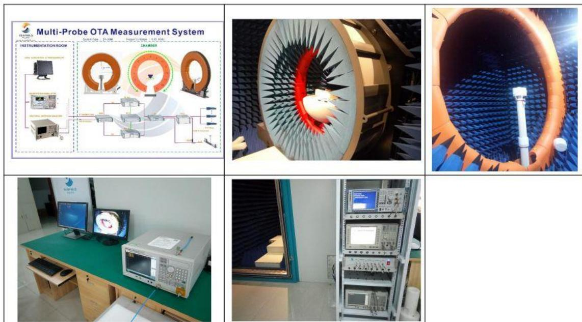
Test system: SY-16M antenna measurement system/SY-24M antenna measurement system
