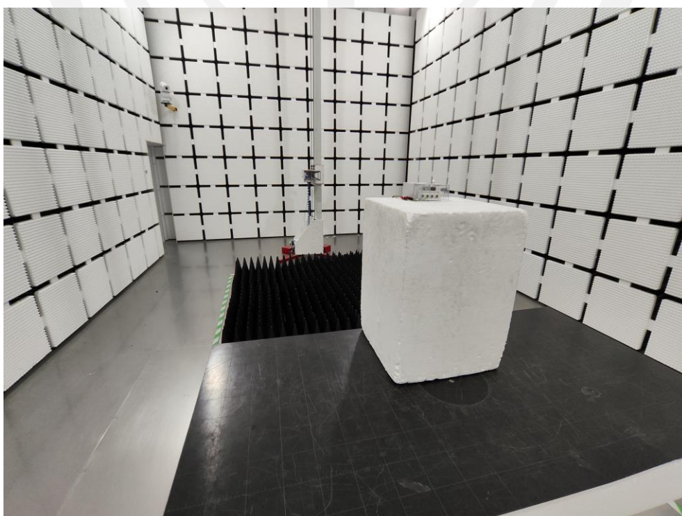
Spurious Radiation Emissions Test (>1G)
