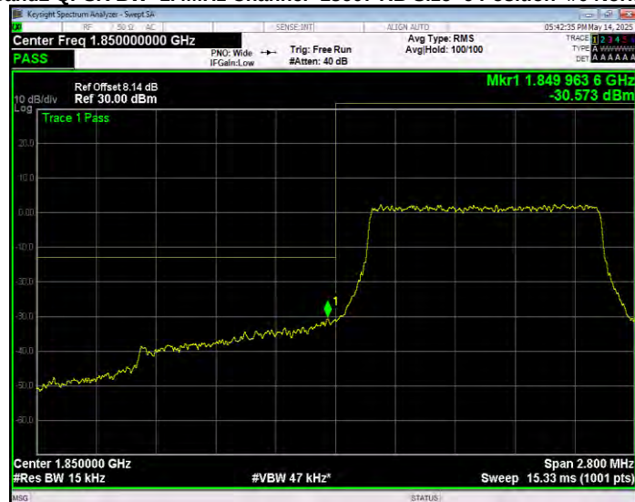
Band2 QPSK BW=1.4MHz Channel=18607 RB Size=6 Position=#0 Normal
