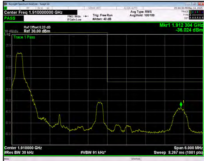
Band2 QPSK BW=3MHz Channel=19185 RB Size=1 Position=#0 Normal
