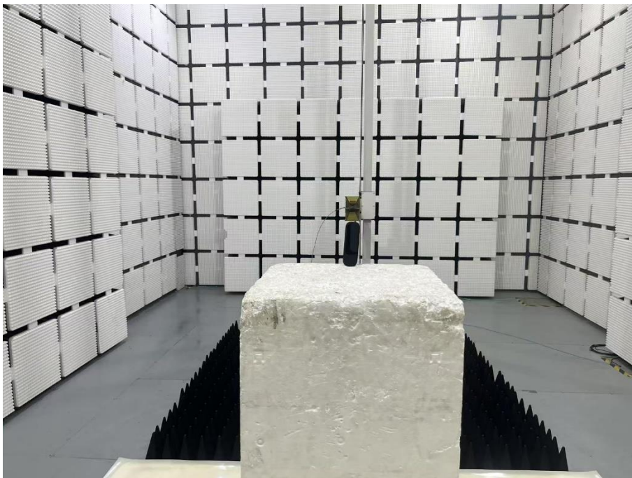
Set-up for Radiated Spurious Emission, Above 1GHz
