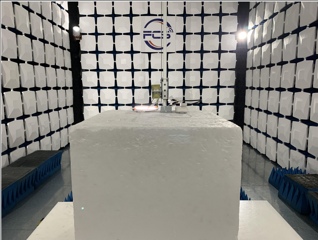
Above 1GHz for radiated emission test setup
