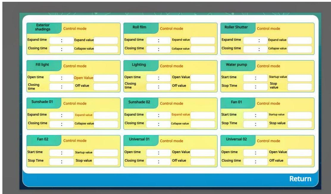
① Set the automatic control mode for external shading
