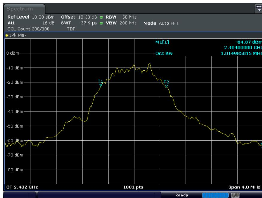
**B.1. Middle Ch. (2.440 MHz)\_6dB Bandwidth**
