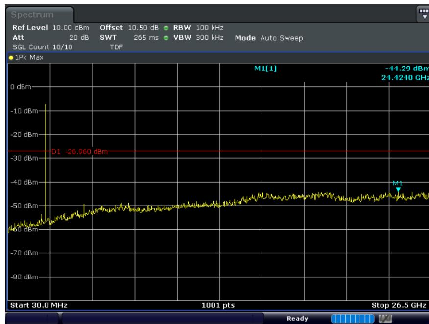
**B.1. Middle Ch. (2 440 MHz)\_Spurious emissions**
