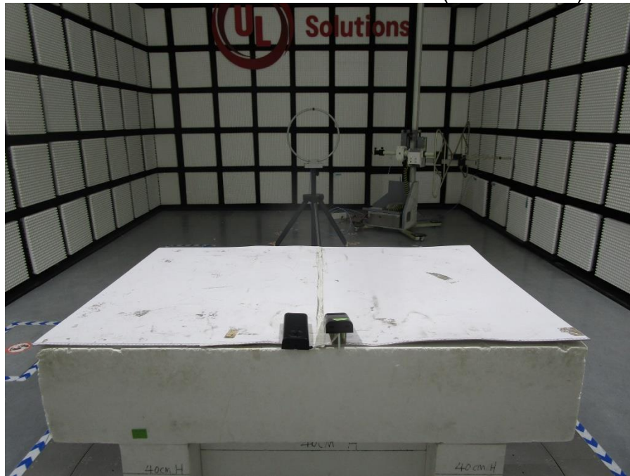
POWERLINE CONDUCTED EMISSIONS MEASUREMENT SETUP
