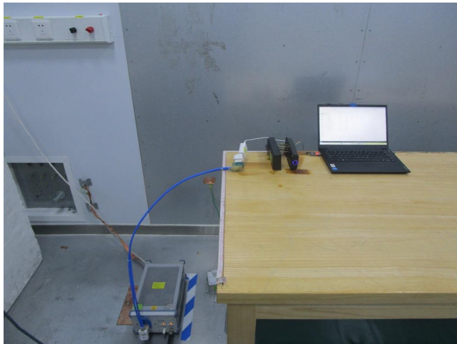
POWERLINE CONDUCTED EMISSIONS MEASUREMENT SETUP
