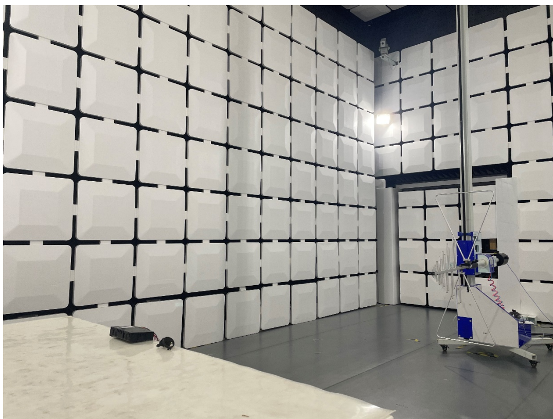
Description: Radiated Emission Test Setup for 30MHz-1GHz
