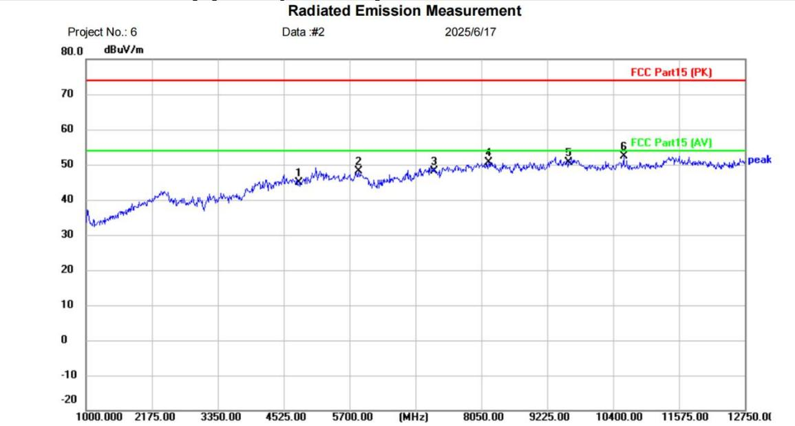
Site: Limit: FCC Part15 (PK) EUT: Bluetooth module M/N: RF06 Mode: BLE1M TX 2402 Note: Polarization: **Vertical** Power: Temperature: (C) Humidity: %RH
