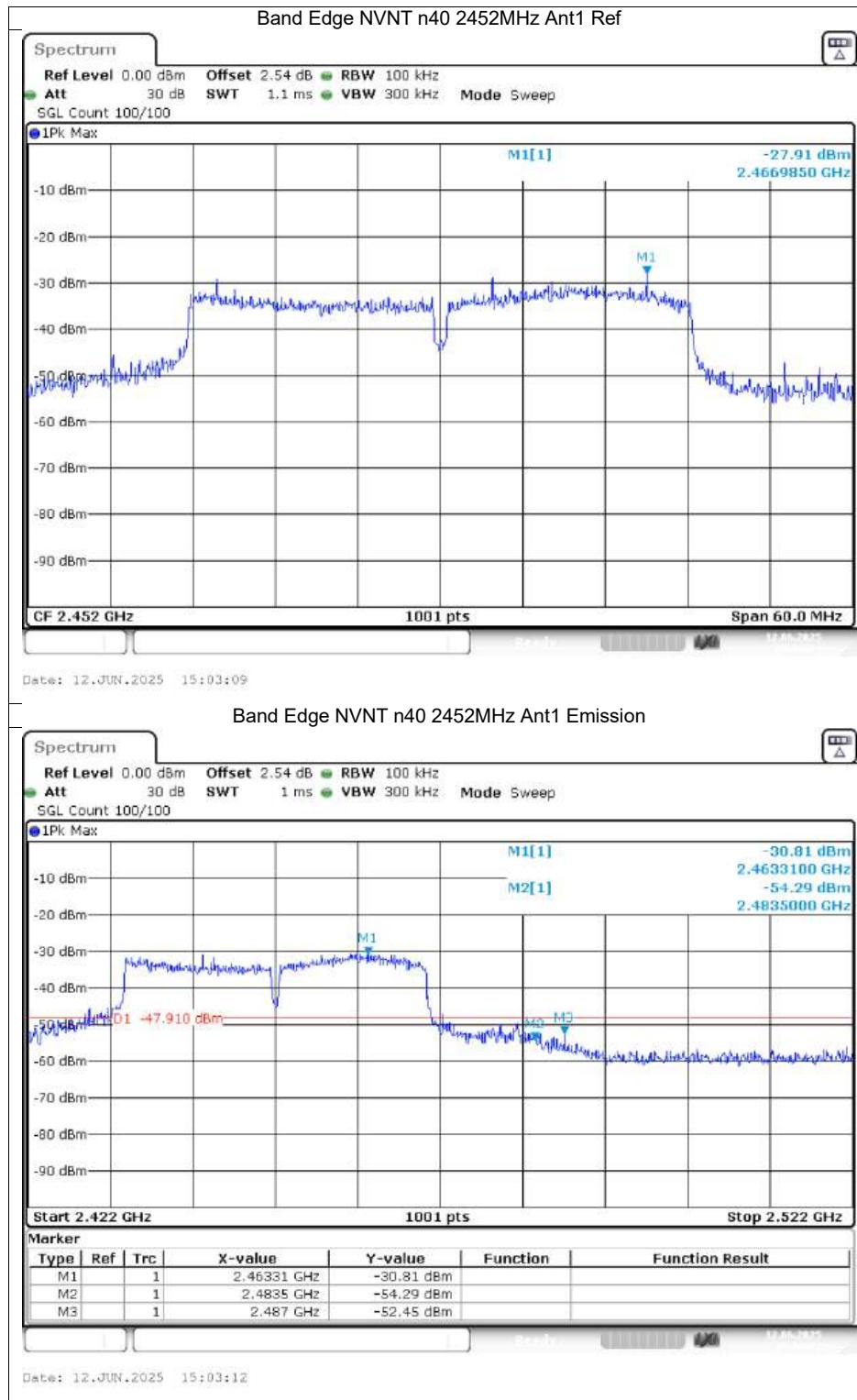
Note: The tests were conducted across frequencies from 9 kHz to 2.4 GHz. However, for frequency points below 2327 MHz, the emission levels were too low (below 20 dB), so the test plots for these frequencies were not included.
