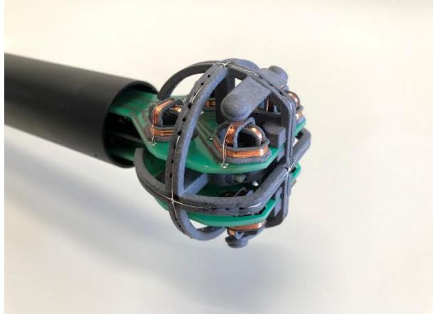
Test probe, without the casing
